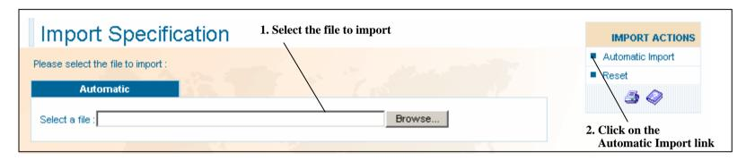
When the user clicks on the "Automatic Import" link, the notepad import screen is displayed (see below). The file selected can have two different structures depending on the import method used. Notepads can be imported using two different methods: "fixed length file" or "separator file".
